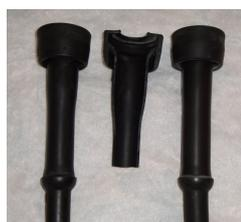
Liner comparison: Same liner, two on left used with short C Phase machine, liner on right used on conventional C phase machine
